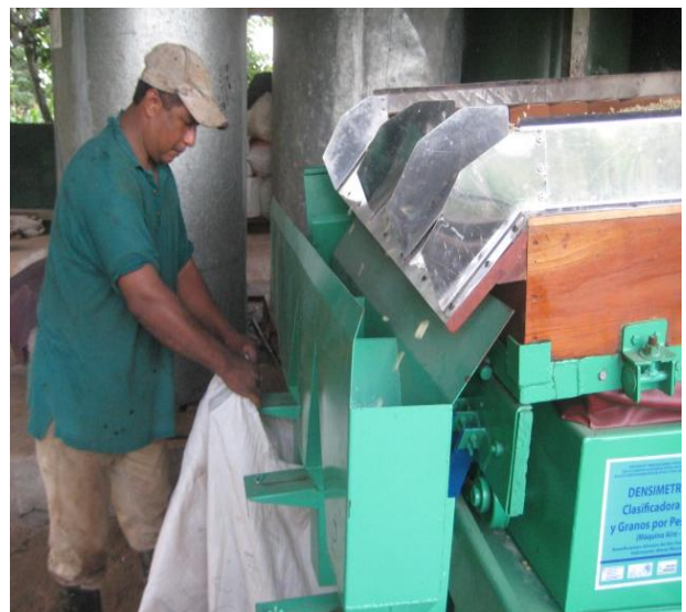
Figure 2. Alfredo Estrada operating the newly acquired gravity mill used to grade seed.
